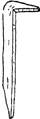
HOOP NAIL for fixing barrel hoops
