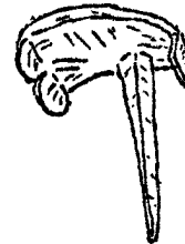
TENTER HOOK the means of holding cloth stretched on tenter frames
