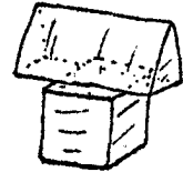
FROST COGS & FROST NAIL screw type frost cogs may be detached from the horseshoe after icy weather, the riveted kind are permanently attached with the shoe. Frost nails serve as a means of attaching the shoe as well as gripping the road
