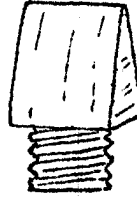
FROST COGS & FROST NAIL screw type frost cogs may be detached from the horseshoe after icy weather, the riveted kind are permanently attached with the shoe. Frost nails serve as a means of attaching the shoe as well as gripping the road
